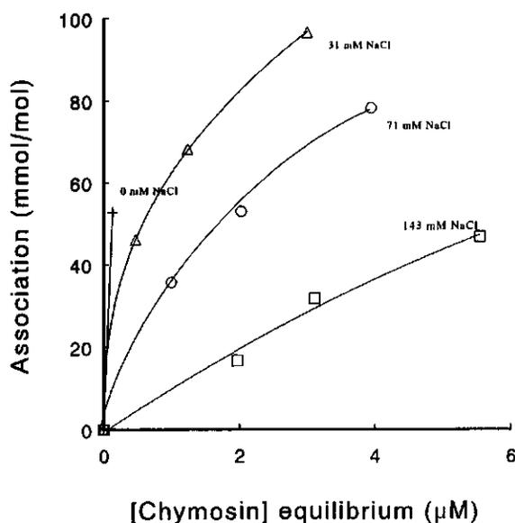
**Figure 5.** Effect of ionic strength on the association of chymosin with para- $\kappa$ -casein (mmol chymosin/mol para- $\kappa$ -casein) in a solution of 1.0 g  $\kappa$ -casein/l in 0.01 M imidazole-HCl buffer. pH 6.3, 30 °C. Amount of NaCl added is indicated.  $I=8$  plus amount of NaCl added (mM).
