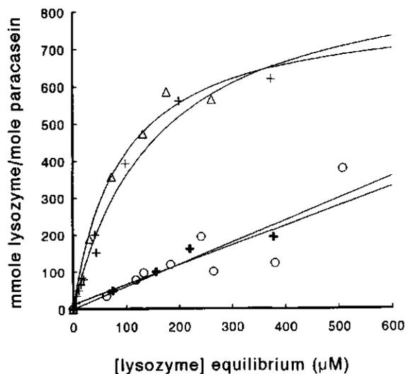
*Fig. 3 Adsorption isotherms showing the lysozyme-para-casein association (mmol/mol) as a function of [lysozyme] in the supernatant of the milk at pH 6.0 and 30 °C. Artificial casein micelles: whole caseinate (+), whole caseinate three times diluted ( $\Delta$ ),  $\beta$ : $\kappa$ -casein 1:2 ( $\circ$ ) and  $\beta$ : $\kappa$ -casein 1:2 three times diluted (\*).*
