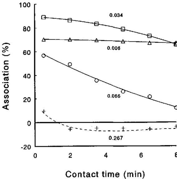
**Figure 1.** Association of chymosin with para- $\kappa$ -casein (in % of total chymosin) as a function of time after addition of chymosin to solutions of  $\kappa$ -casein. pH 6.3, 30°C, ionic strength 0.06 M (20 mM NaCl added). Concentrations of  $\kappa$ -casein (g/l) and chymosin ( $\mu$ M): 3.3 and 5.71 ( $\square$ ); 1.0 and 0.31 ( $\Delta$ ); 1.0 and 3.37 (o); 0.15 and 2.05 (+), respectively. The ratio of chymosin to  $\kappa$ -casein (mol/mol) is indicated.
