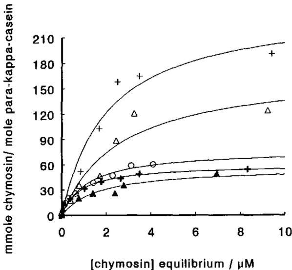
Fig. 5 The influence of the  $\kappa$ -casein concentration, in various dilutions of the soya-oil/ $\kappa$ -casein emulsions, on the association with chymosin after 20 min of incubation in 25 mM K-phosphate buffer pH 5.5 at room temperature. Emulsion dilution:  $10 \times$  (+),  $5 \times$  ( $\Delta$ ),  $2 \times$  (o),  $0 \times$  (+) and  $0.5 \times$  ( $\blacktriangle$ ).
