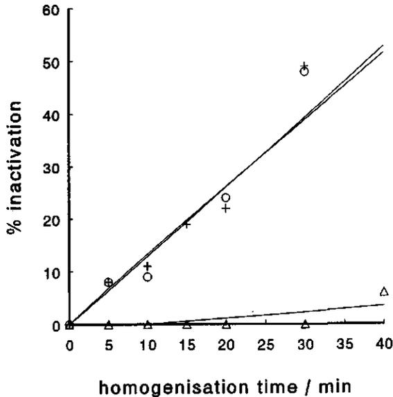
*Fig. 1. The influence of number of homogenization head passages and foam formation during homogenization on the inactivation of chymosin (0.66  $\mu$ molar chymosin, pH 5.8, 50 mmolar K-phosphate buffer). Loss of chymosin activity in the solution during foam development (O) , in the foam itself (+) and in the solution when foam was not allowed to form ( $\Delta$ ) .*
