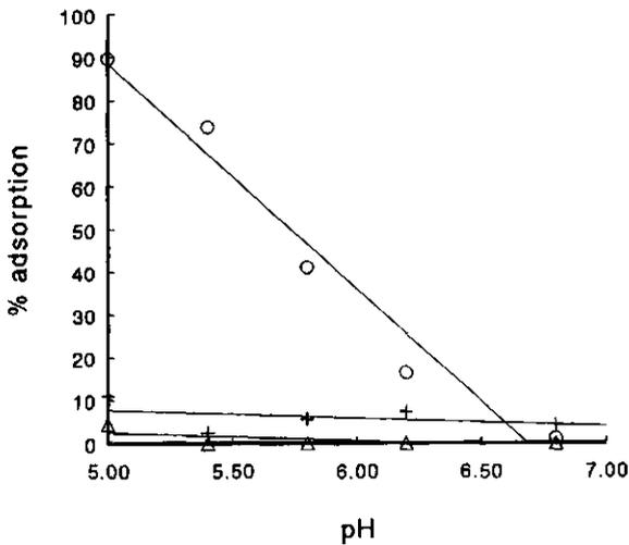
*Fig. 1 The association of chymosin in % of initial amount of chymosin (0.7  $\mu$ molar) with adsorbed  $\alpha_s$ -casein (+),  $\beta$ -casein ( $\Delta$ ) and  $\kappa$ -casein (o) as a function of pH, after 20 min of incubation at room temperature in 25 mM K-phosphate buffer.*
