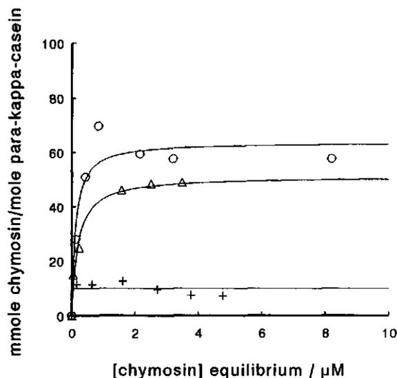
Fig. 4 The influence of temperature on the association of chymosin with  $\kappa$ -casein adsorbed onto soya-oil emulsion droplets, after 20 min of incubation in 25 mM K-phosphate buffer at pH 5.5. 4 °C (o), 20 °C ( $\Delta$ ) and 40 °C (+).
