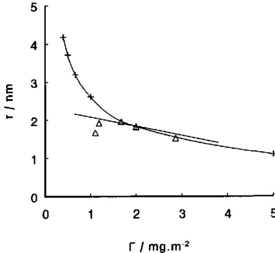
Fig. 2. Calculated radius of lysozyme molecules adsorbed onto an air/water ( $\Delta$ ) and an oil/water (+) interface as a function of surface load  $\Gamma$ . After refs. [22], [23].
