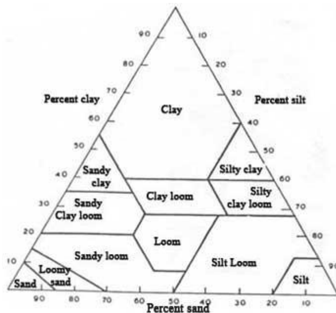
Figure A2.1 Soil triangle. Relationship between contents of clay, silt and sand in determining the different kinds of soil
