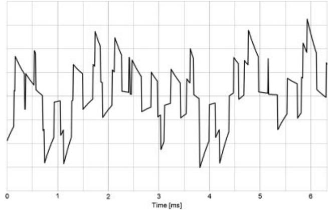
Fig. 1. Immuent signal shape when adapted for a coil with resistance  $R$  being 400 times the self-inductance  $L$  of the coil. The time given at the x-axis (in ms) starts 1 ms after the four signal components start all in phase. The signal has a non-repetitive character and sharp edges. The scale of the y-axis is arbitrary.
