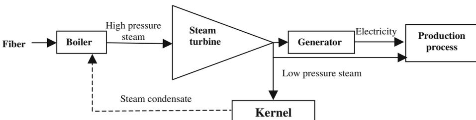
Figure 5. Recycling of condensate to boiler.
