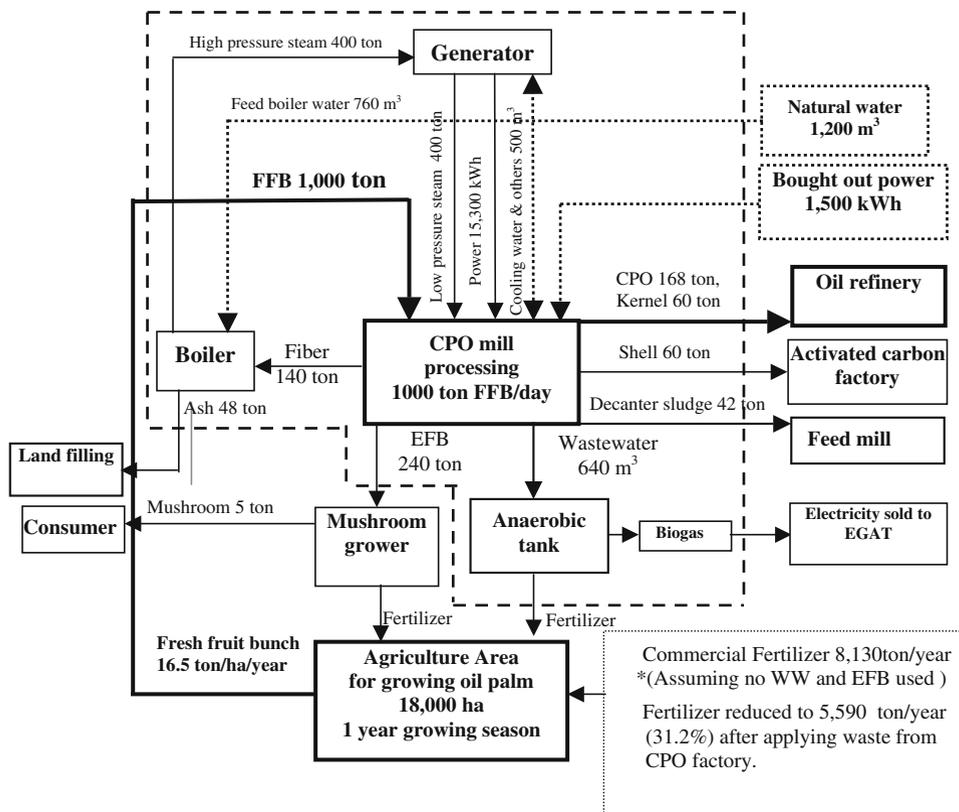
Figure 7. Material balance of the proposed physical–technological model of a CPO industrial ecosystem with a minimum waste. —, Production line; - - -, Boundary of CPO; ·····, Factory; —, Natural resource input; ·····, Product/by-product/waste.
