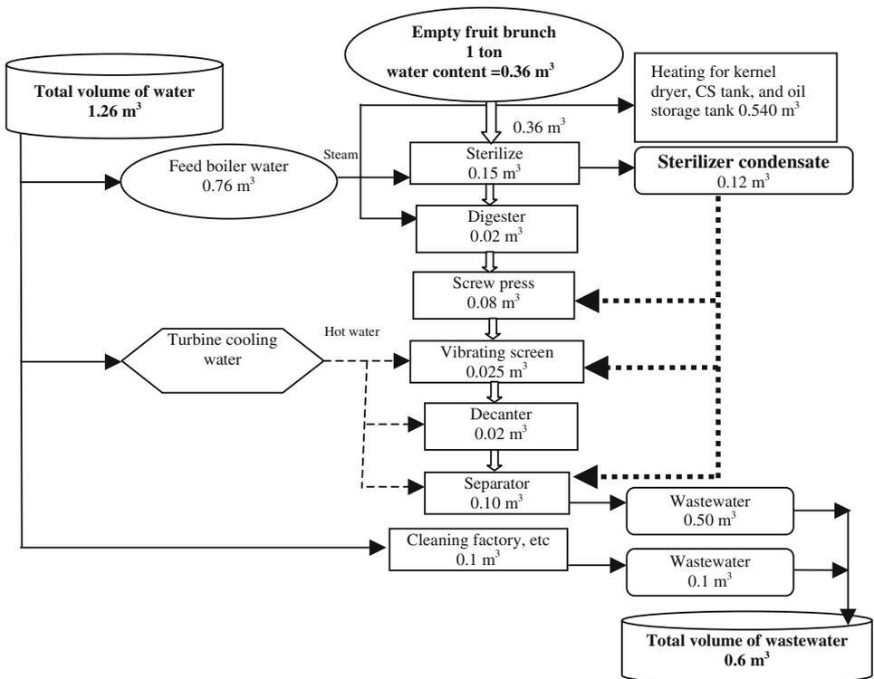
Figure 4. Flow diagram of production process and in-plant water recycles (volume per ton FFB).
