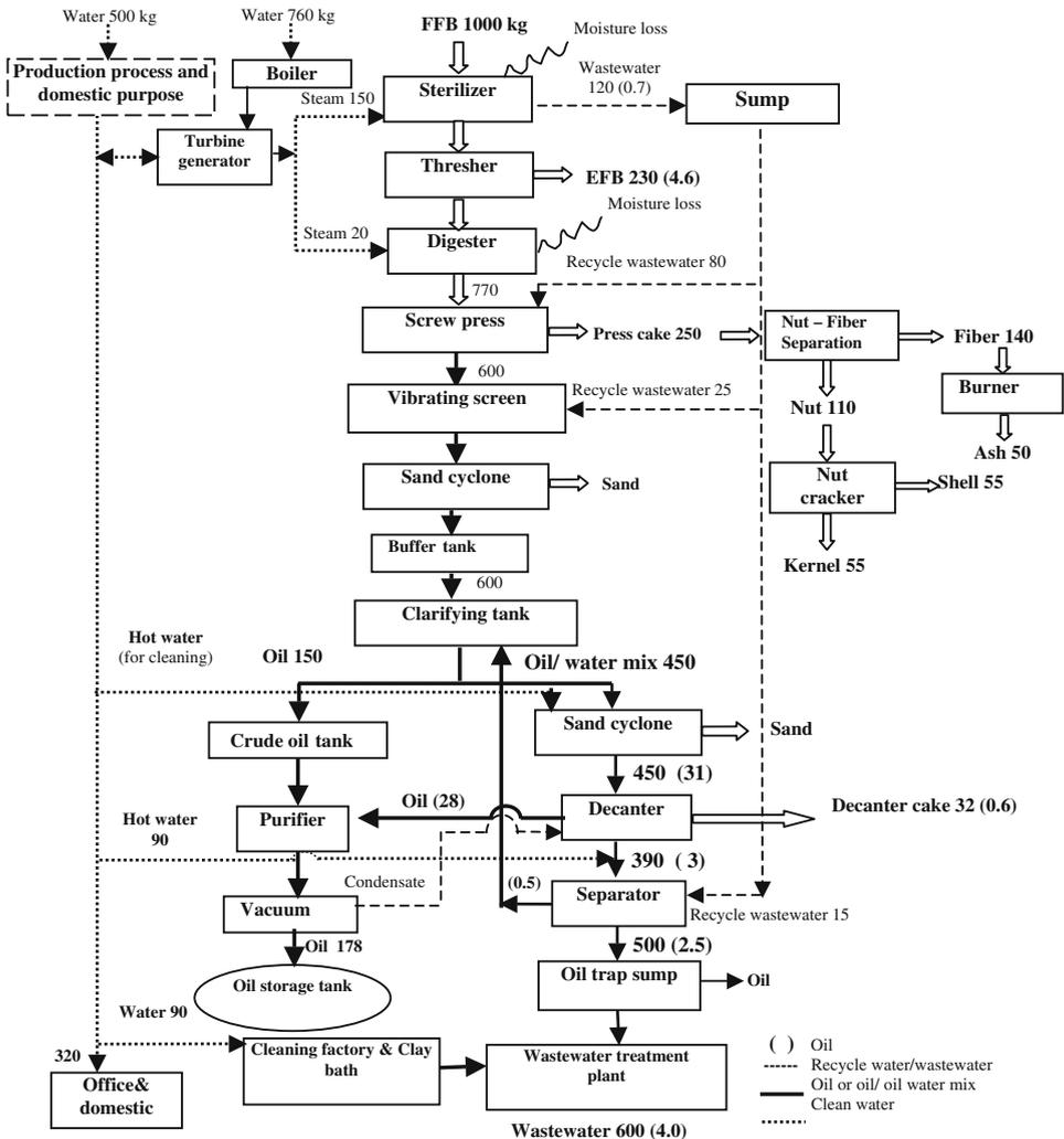
Figure 1. Mass balance (in kg) of production process of a study factory.
