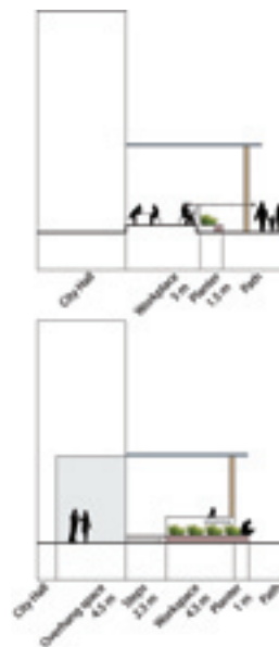
figure 10.25 Cross section of the workplace at Spuiplein (top; view across, bottom; side view).
