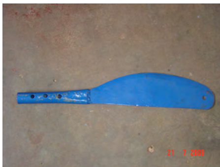
Photo 2.9: Panga with a sickle shaped cutting edge
