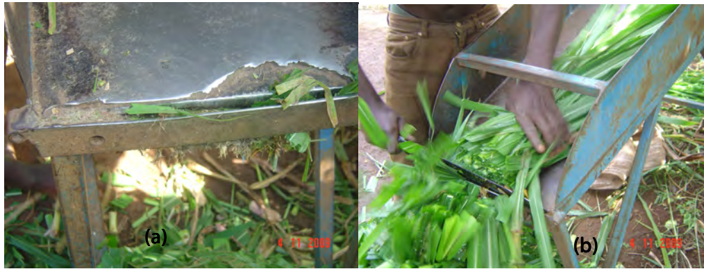
Photo 4.2: Plate controlling length of cut removed
