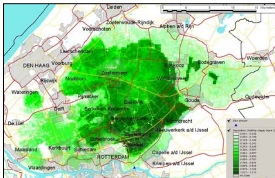
Figure 2. Deposition of sediment during the settling stage, according to the ERA model [ \text{kg/m}^2 ].
