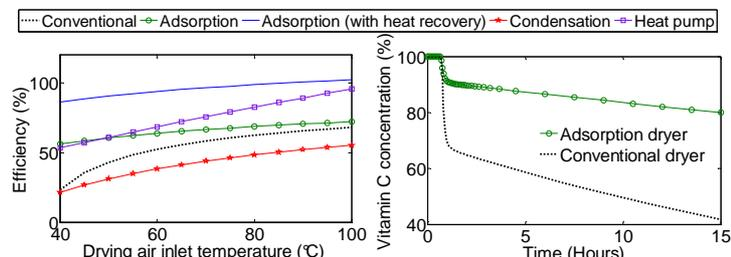
Fig. 6. (a). Energy efficiency of conventional dryer compared with dryers with 50% drying air dehumidification (b). Normalized vitamin C degradation for adsorption & conventional dryer operating at equal energy efficiencies
