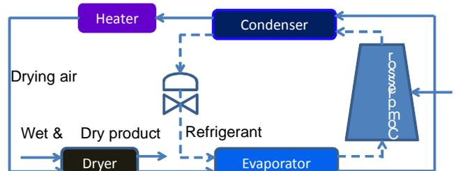
Fig. 4. Heat pump dryer: exhaust air cooled below dew-point and reheated; gained sensible and latent heat "pumped" by compressor
