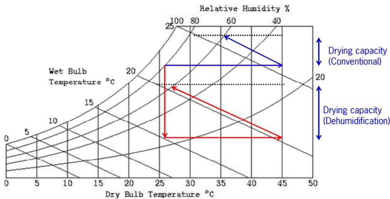
Fig. 1. Psychrometric chart: improved drying capacity by dehumidification
