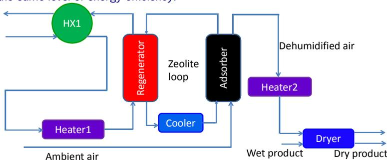
Fig. 2. Adsorption dryer, with regenerator exhaust heat recovery by exchanger HX1
