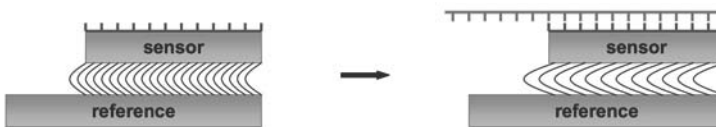
Figure 8. Acoustic detection of increased mass after hybridisation. The frequency of an acoustic wave is altered by increased mass, detected and translated into electrical signal.
