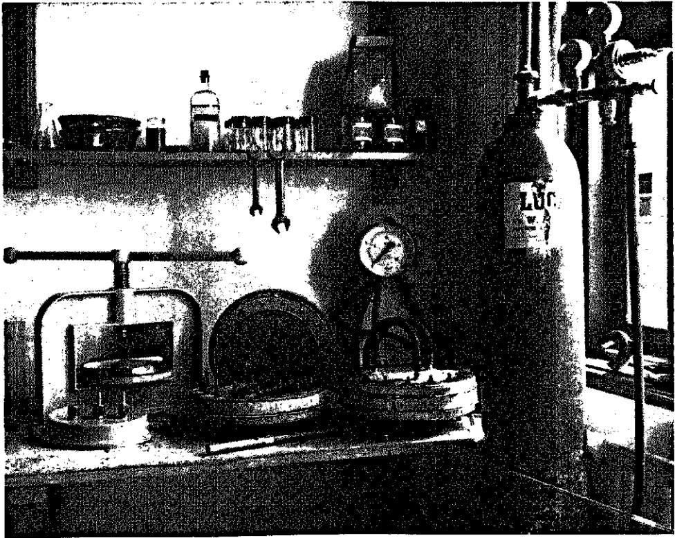
FIG. 20. Pressure membrane apparatus according to RICHARDS for the determination of the moisture retention curve of the soil
