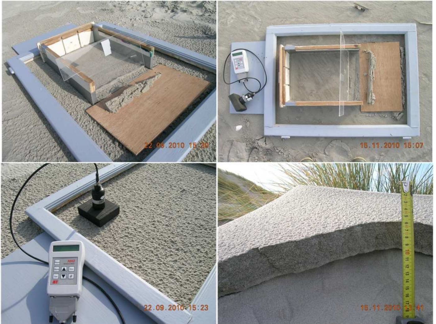
Figure 2. Surface moisture content measurement within a rectangular frame with reference plate
