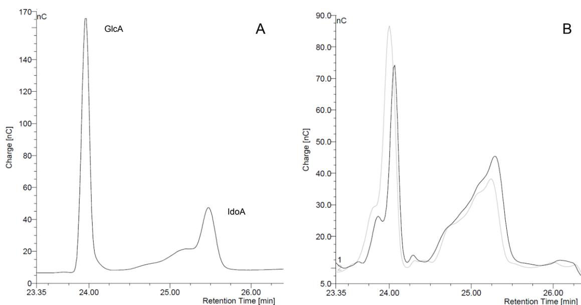
**Figure 3** – Separation of D-glucuronic acid (GlcA) and L-iduronic acid (IdoA) using an HPLC-PAD system. (A) Separation of standards (B) Hydrolyzed (de-O-sulfated) heparin; black = control sample, gray = sample incubated with RED-C5-epimerase.
