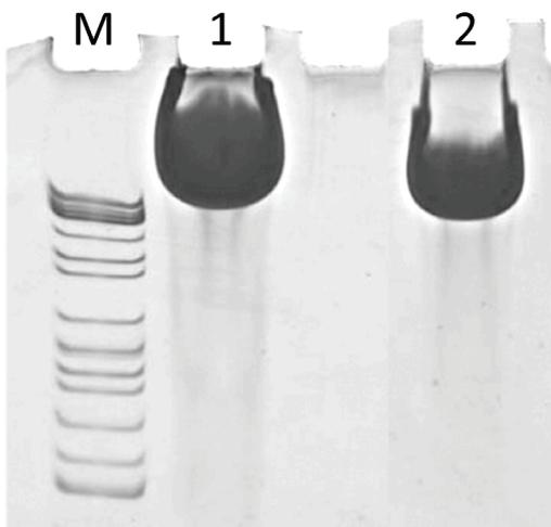
**Figure 6** – TBE-gel based analysis of hyaluronan synthesis by using MBP-PmHAS. Lane M give an indication of the molecular mass. Lane 1 represent hyaluronan production using cell lysate containing MBP-PmHAS, lane 2 represent hyaluronan production by using purified MBP-PmHAS..
