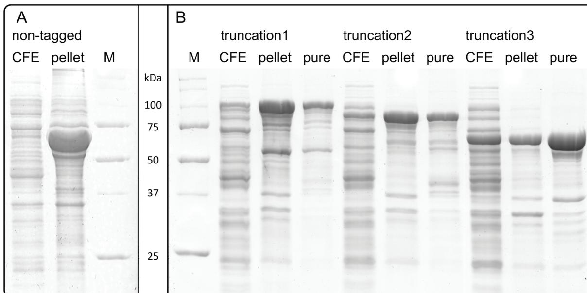
**Figure 4** – Murine D-glucuronyl C5-epimerase production in *E. coli*. (A) Non-tagged C5-epimerase is produced massively (size 67kDa). (B) N-terminal fusion with Maltose Binding Protein (MBP; 43 kDa) results in soluble protein in the cell free extract (CFE). The three N-terminal truncation are 110 kDa (truncation1), 95 kDa (truncation2) and 70 kDa (truncation3) in size.
