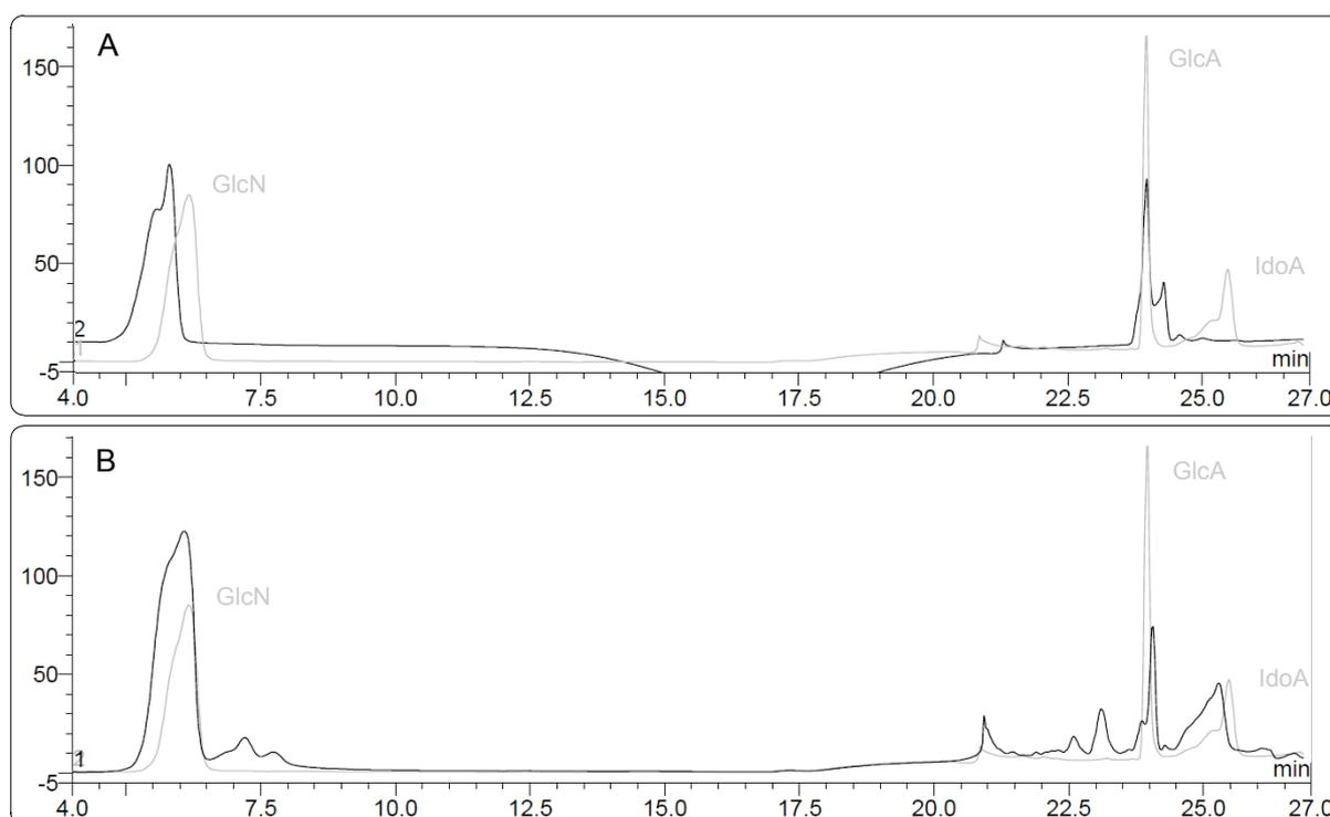
**Figure 2** – Chromatogram HPLC-PAD separation of glucosamine (GlcN), D-glucuronic acid (GlcA) and L-iduronic acid (IdoA). (A) Addition of salt disturbs retention-time of mainly IdoA. (B) Hydrolysis profile of de-O-sulfated (N-sulfated) heparin. Standards are shown in grey, samples are shown in black.
