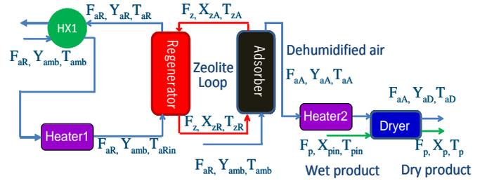
Fig. 1. Adsorption drying system
