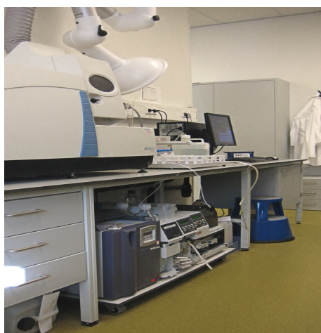
HPLC-ICPMS setup used for speciation.
