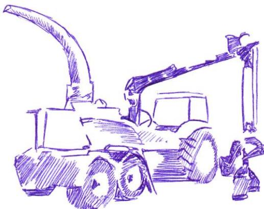
07. Chipper and tractor with crane
