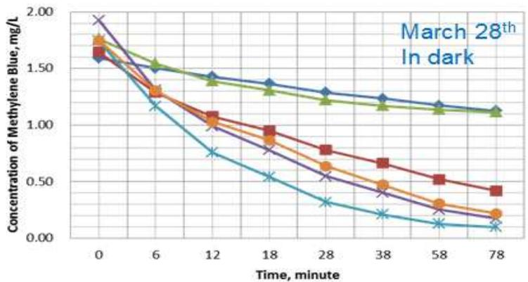
The experiment Decomposition of Methylene Blue with minerals and aeration without exposed to lamp
