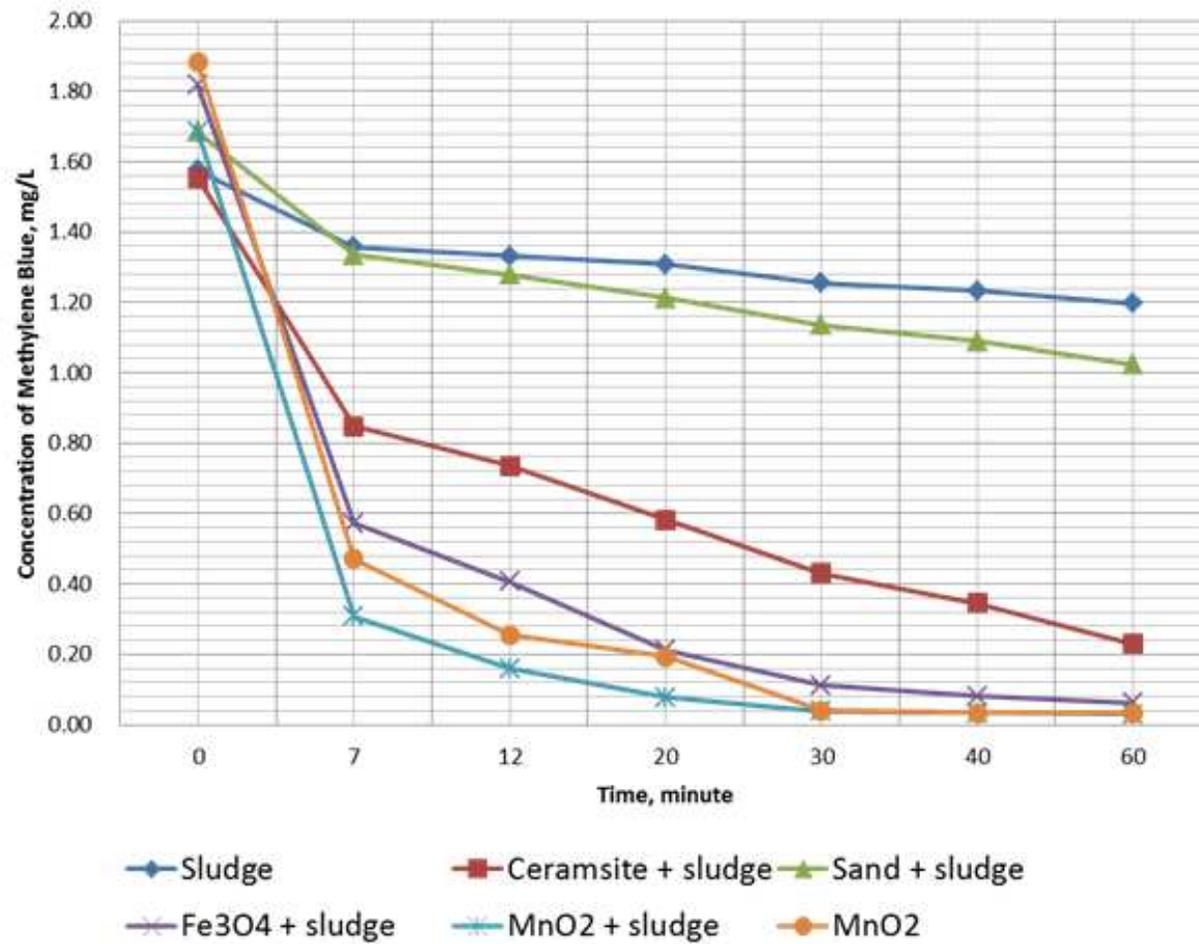
The experiment Decomposition of Methylene Blue with minerals and aeration with exposed to lamp
