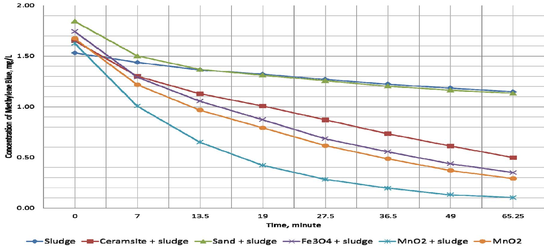
Figure 3 result of the Decomposition of Methylene Blue with minerals and aeration
