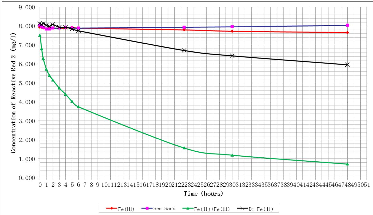
Figure 5 result of the Decolorization of Reactive red 2 at the surface of Magnetite without aeration
