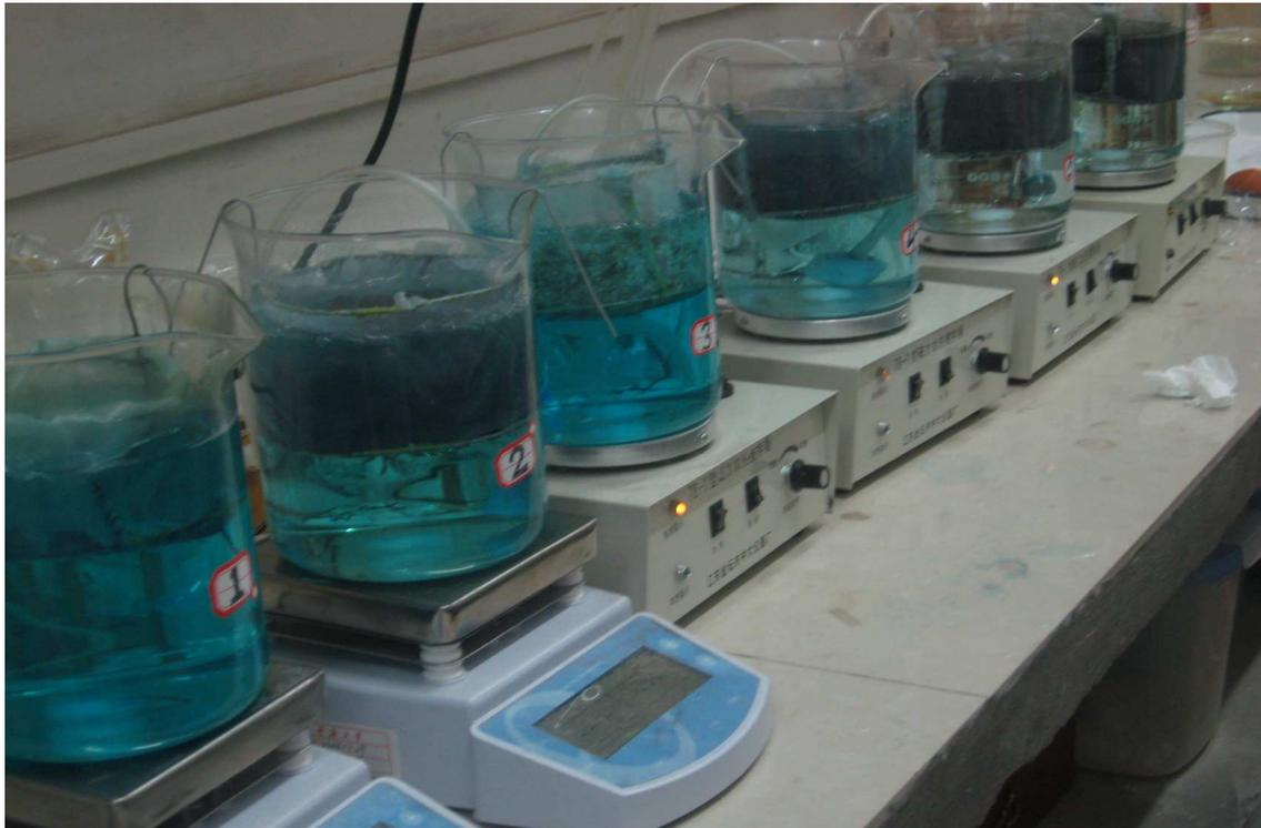
Figure 2 Decomposition of Methylene Blue with minerals and aeration
