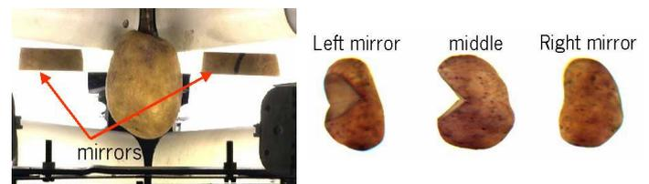
Figure 3. Camera view of the potato as it passes the gap between the conveyors (left). The produced images are sent to the DSP's for processing (right).
