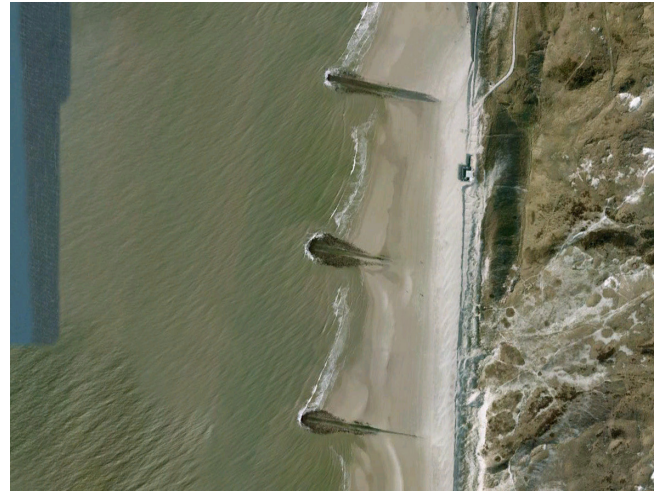
Dams closer to each other tend to catch and hold more sand
