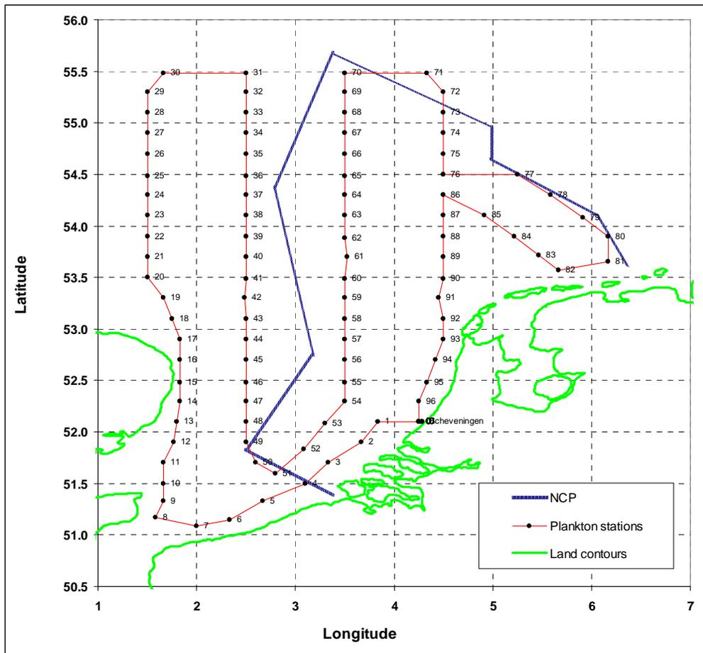
Figure 3. Initial survey grid consisting of 96 stations. This grid can be sampled in 5-6 days (from 8:00am on Monday to 9:00am on Saturday) if an overall speed of 11 knots is achieved.
