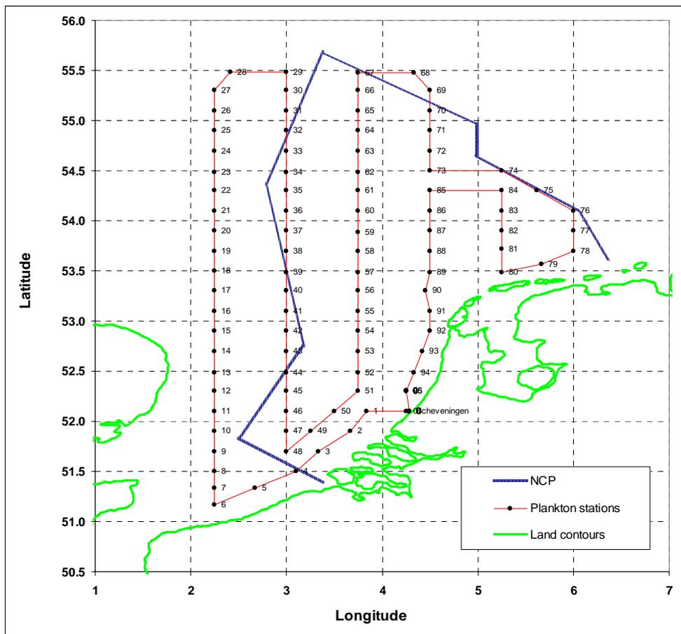
Figure 9. Survey grid consisting of 95 stations in which the spatial coverage is reduced and the spatial resolution is increased compared to the original survey grid (Figure 3). This grid can be sampled in 5-6 days (from 8:00am on Monday to 3:00am on Saturday) if an overall speed of 11 knots is achieved.
