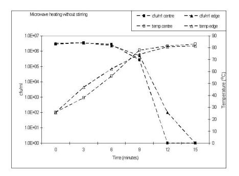
*Figure A4.4 Survival of* C. perfringens *in and temperature of pea soup during heating in microwave oven without regular stirring Measurement of temperature of the soup in two places, centre and edge of the bowl.*
