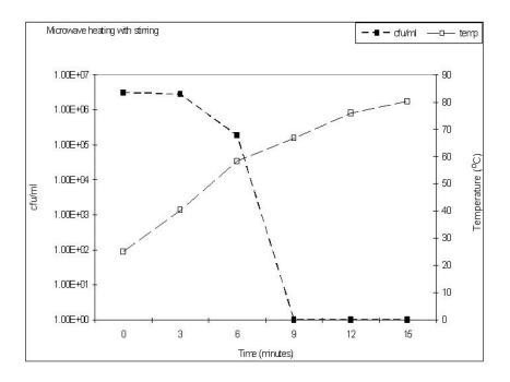
*Figure A4.3 Survival of* C. perfringens *in and temperature of pea soup during heating in microwave oven with regular stirring*
