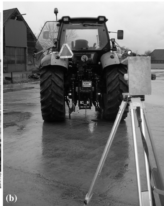
Figure 3. Precision positioning used to acquire field geometry (a) and to check communication with farm equipment (b).
