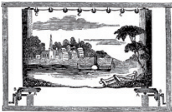
Figure 1.4: Diagram showing the mechanism of a moving panorama, from Scientific American , 1848
