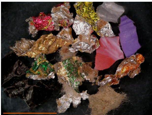
Figure 6 and 7. Presumed remnants of packaging materials in a cocoa products and in a sweet syrup. Bar in lower left corner is 1 cm. Figure 6 (left): aluminium foil and plastic; complete overview of the recovered material from a sample with a contamination level of 0.2 % w/w. Figure 7 (right): conglomerates of paper fibres collected from a sweet syrup; part of the recovered material from a sample with a contamination level of 0.44 % w/w.
