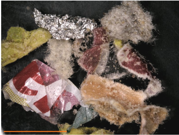
Figure 4 and 5. Presumed remnants of packaging materials in bakery products. Bar in lower left corner is 1 cm. Figure 4 (left): mixture with aluminium particles, paper and printed foil; complete overview of the recovered material from a sample with a contamination level of 0.21 % w/w. Figure 5 (right): pieces of plastic clips among other particles; complete overview of the recovered material from a sample with a contamination level of 0.05 % w/w.
