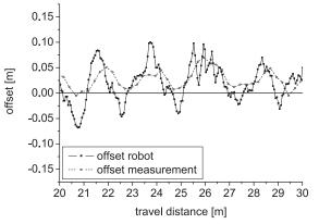
Figure 5. Position accuracy of the WURking robot, measured with the ultrasonic sensors of the robot and the measurement device.
