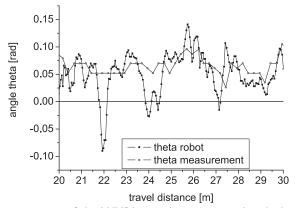
Figure 6. Orientation accuracy of the WURking robot, measured with the ultrasonic sensors of the robot and the measurement device.
