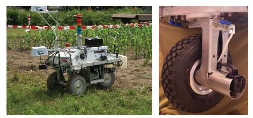
Figure I. The WURking robot (left) and one of the wheel units (right).
