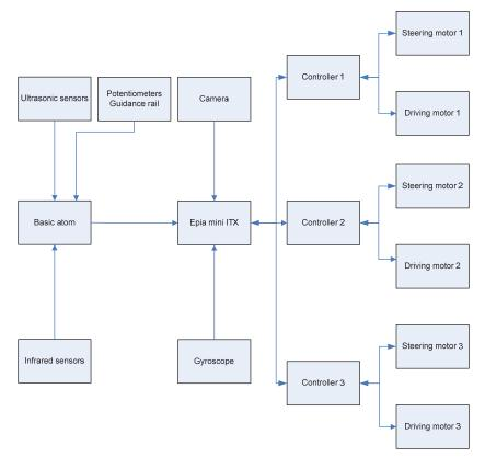
Figure 2. Schematic diagram of the different components of WURking.
