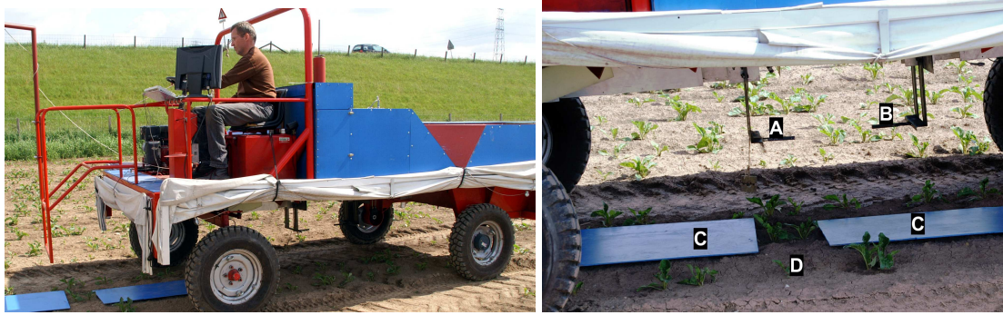
Figure 1 InspectorMobile measurements in sugar beet field. A and B are reflectance references in the field of view of sensor 1 and sensor 2 respectively. C are plastic sheets covering vegetation that was not recorded. D is one of the plants recorded by sensor 1.
