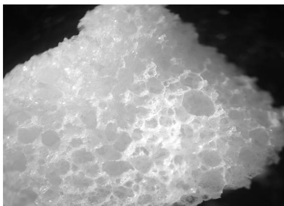
Fig. 1. Glass foam granulate magnified 40×. Fig. 2. Healthy roots, branching into hair roots above the water level.
