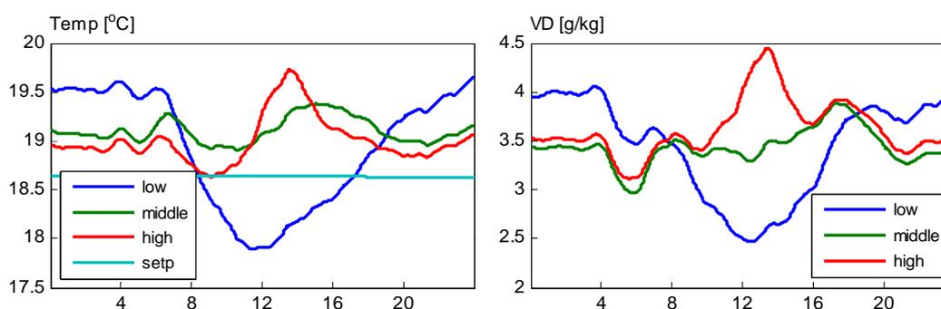
Fig. 3. Cyclic temperature (left) and vapor deficit (right) of grower 7 from 1 till 31 May 2009.
