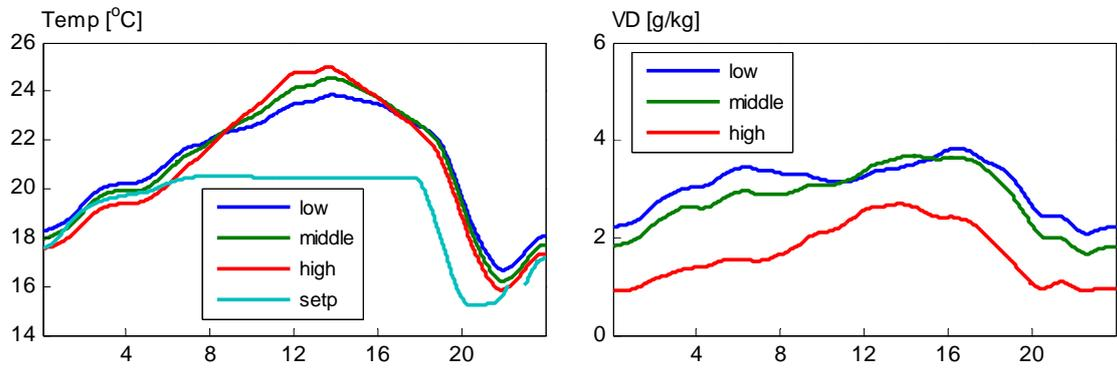
Fig. 5. Cyclic temperature (left) and vapor deficit (right) of the conditioned compartment of grower 2 (Table 1) from 1 till 31 May 2009.
