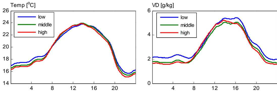
Fig. 6. Cyclic temperature (left) and vapor deficit (right) of the conventional controlled compartment of grower 2 (Table 1) from 1 till 31 May 2009.
