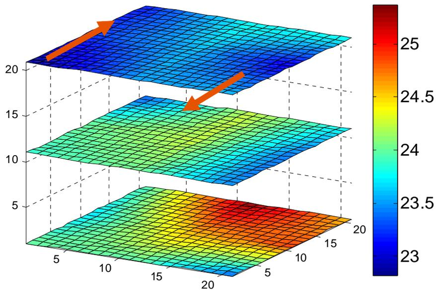
Fig. 6. Temperature profile during cooling periods (between 25 July and 1 August 2008) for a repeatable section of a greenhouse at three heights where top coolers are used to condition the air.
