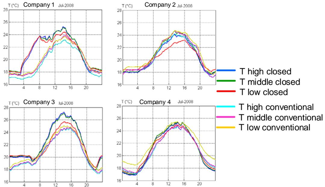
Fig. 2. Temperature at three different heights in the semi-closed greenhouse and the conventional greenhouse at four companies on a 24 hours cycle mean averaged period for the month July 2008.
