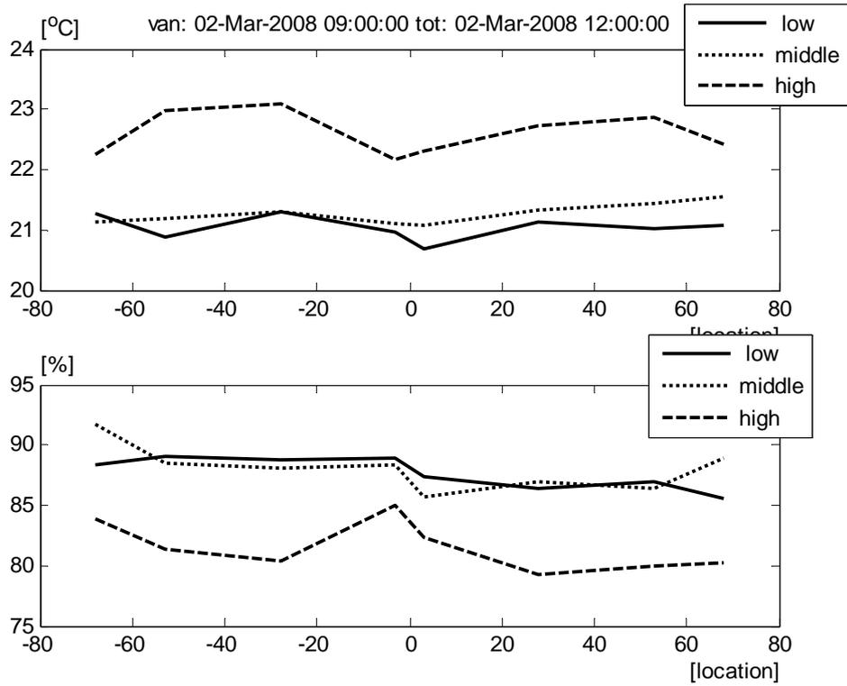
Fig. 5. Temperature and relative humidity profile along the air duct from side to side in the greenhouse during a cooling period.
