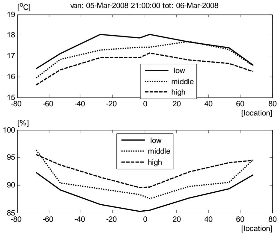
Fig. 4. Temperature and relative humidity profile along the air duct from side to side in the greenhouse during a heating period.
