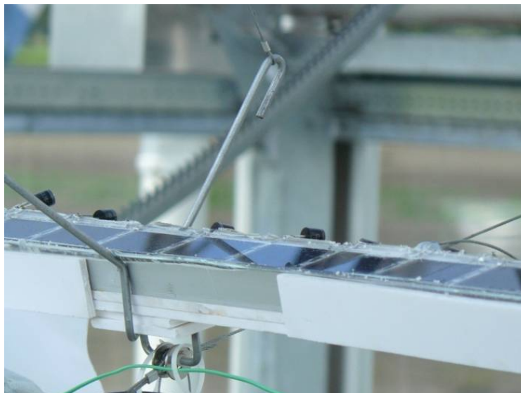
Fig. 6. The TPV module of the system with the silicon cells inside the greenhouse.
