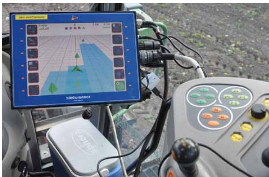
GPS systems are important to precision sowing and weeding
