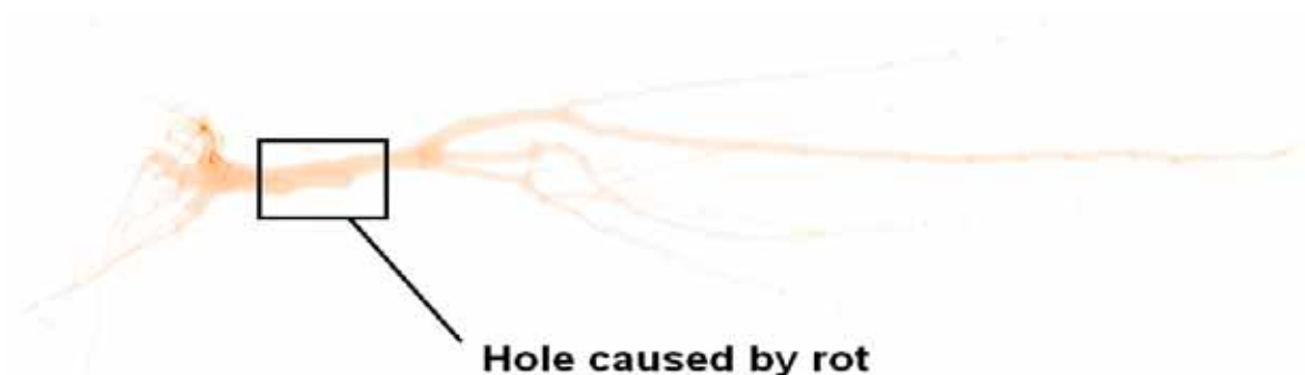
Fig. 15. X-ray image of an intact maple tree marked as suspicious. After destructive assessment of this tree, the hole turned out to be caused by rot.
