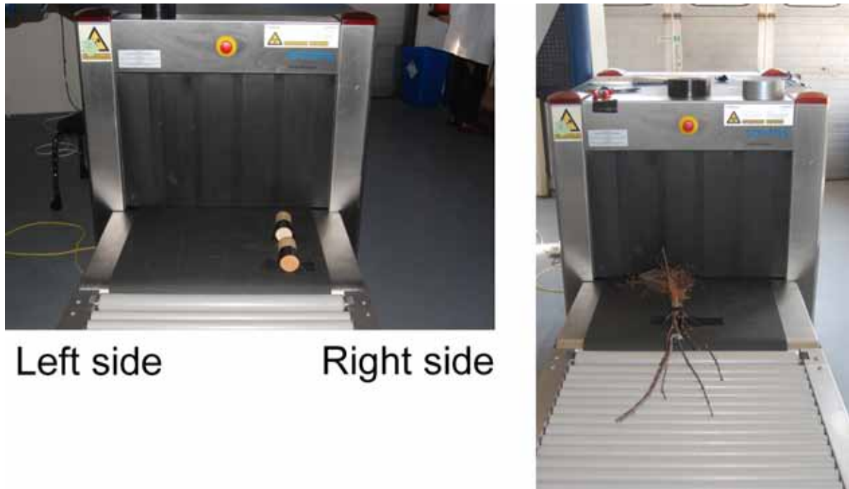
Fig. 3 X-ray inspection system with a pre-drilled wooden axles or an intact tree fixed on the conveyer by tape
