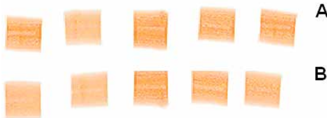
Fig. 10. The effect of boredust on the visual appearance of boreholes in X-ray images. Images are retrieved from maple stems with outer diameters of 30-35 mm containing pre-drilled holes of 5 mm: A) holes without boredust, B) same stems but holes filled with boredust
