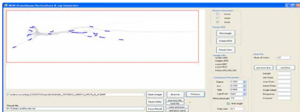
Fig. 17. Detection of a hole caused by rot by machine vision. Besides this hole, also 16 holes were recognised which were actually no holes.
