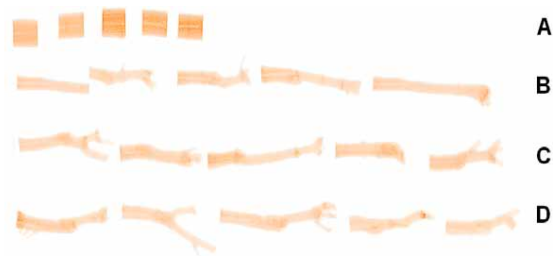
Fig. 13. The effect of stem diameter, pre-drilled hole diameter and hole position on the visual appearance of boreholes in X-ray images. A) d_{out} = 30-35 \text{ mm} , d_{hole} = 5 \text{ mm} , State = A; B) d_{out} = 20-25 \text{ mm} , d_{hole} = 5 \text{ mm} , State = A; C) d_{out} = 20-25 \text{ mm} , d_{hole} = 3 \text{ mm} , State = A; D) d_{out} = 20-25 \text{ mm} , d_{hole} = 5 \text{ mm} , State = D.
