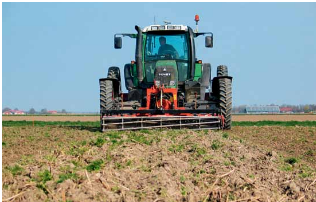
Tractor with adjusted wheel distance (3.15 m) for BASIS
