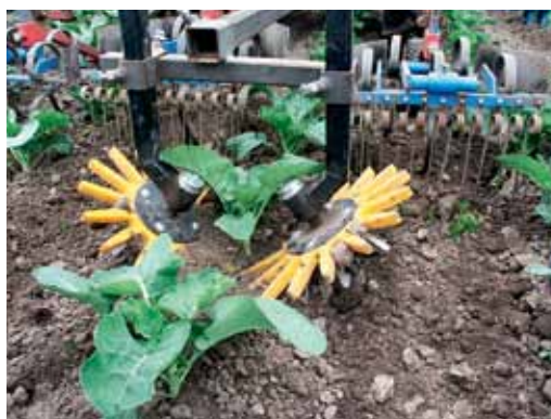
The finger weeder controls weed in the crop row
