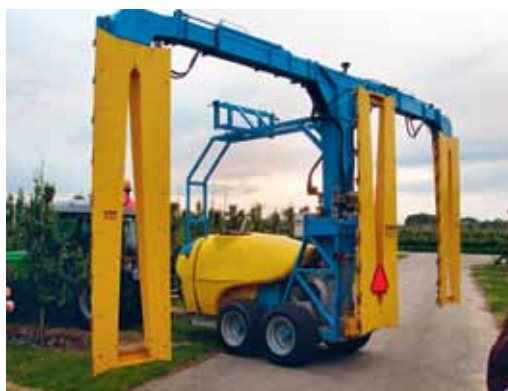
Demonstration of the three-row low-emission KWH sprayer
