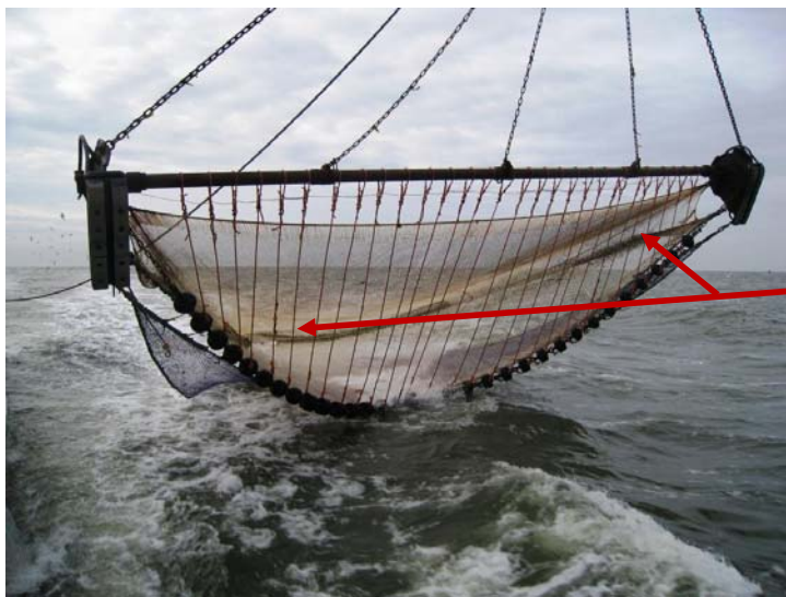
Figure 5. Picture of the letterbox with guiding panel; red arrows point to the guiding panel (schotje) and the release hole (brievbus).
