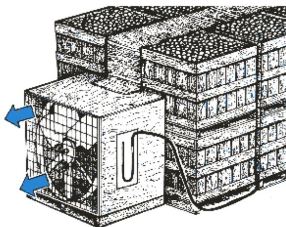
Figure 2: Fan and pallet bin arrangement used to dry onions.
