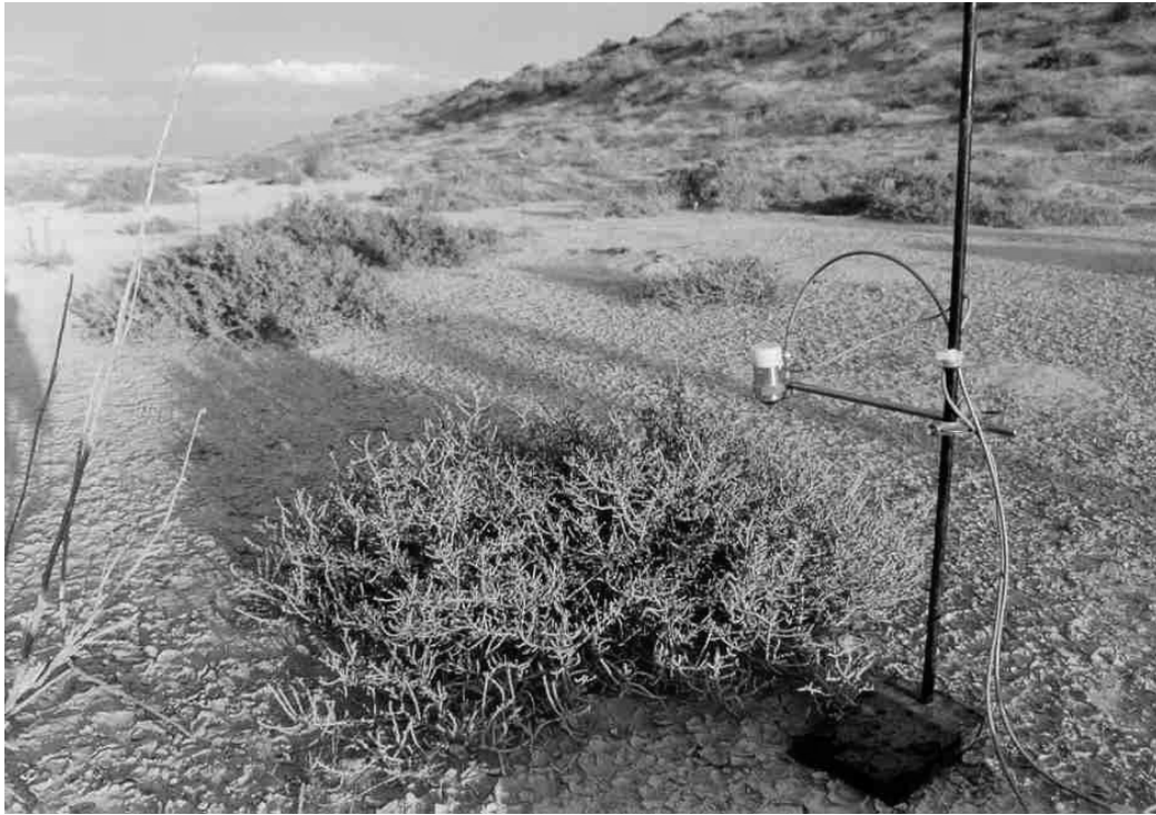
Figure 4.10: Optical Wetness Sensor installed above an Anabasis articulata plant.
