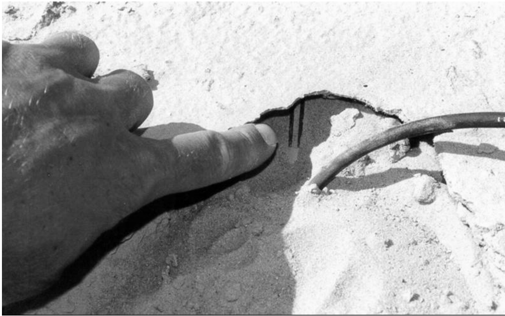
Figure 5.3: Placement of a relative humidity probe underneath the crust
