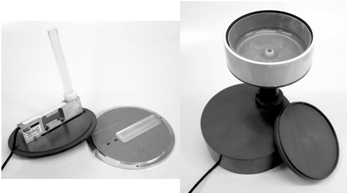
Figure 3.2: Left panel: Load Cell affixed to a PVC base plate. An aluminum base plate option is also shown (note the depression to allow the Load Cell to bend). Right panel: Microlysimeter showing the empty plastic sampling dish and protective cover for rain or storage.
