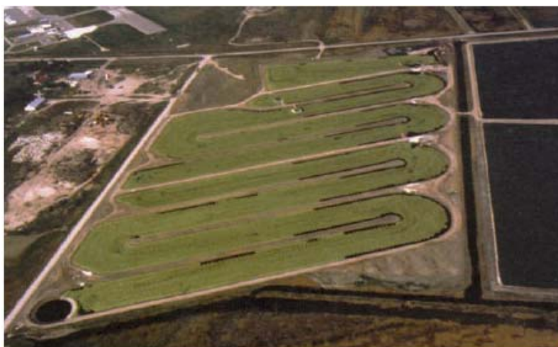
Photograph 2: Duckweed-covered serpentine plug-flow lagoon in the USA for tertiary treatment of effluent from three facultative lagoons followed by a wetland buffer. Design flow is reported at 19,000 m 3 /d, with peak flows reaching 38,000 m 3 /d. (Photograph: Lemna Corp. 1994).
