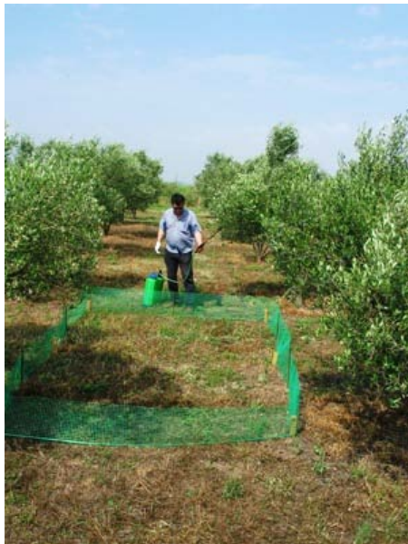
Figure 5-3 Experimental design for testing treated wastewater application on soil water repellency. Photo: Vasilis Diamantis.
