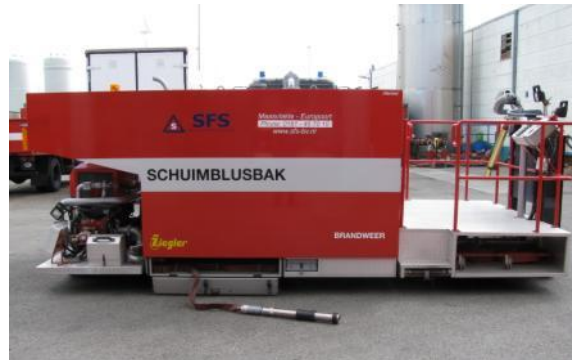
Integrated foam mixing and pumping unit
