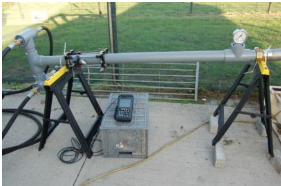
Figure 18 Gas flow meter and improved manifold
