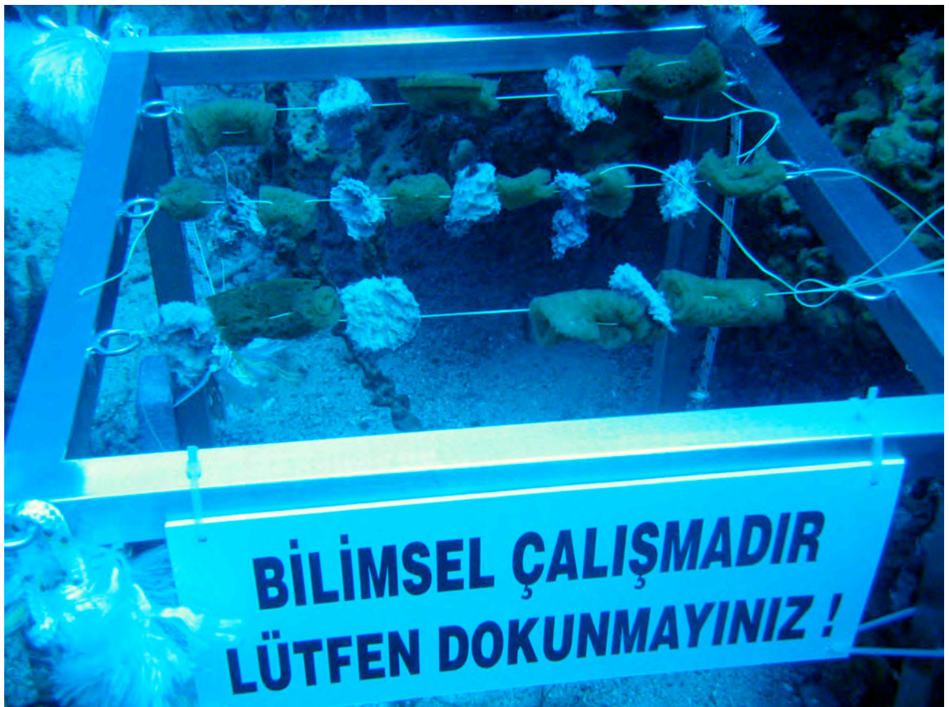
Fig. (1). Stainless steel frame hosting ten explants of D. avara .
