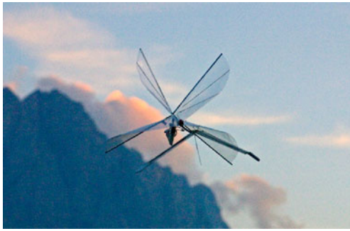
Fig. 1 DelFly, a flapping wing micro aerial vehicle inspired by insect flight with slack sail-like wings [3]
