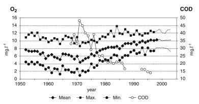
Figure 3. Yearly average, minimum and maximum observed dissolved oxygen concentrations, and yearly average of the COD in the river Rhine measured at the German–Dutch border.
