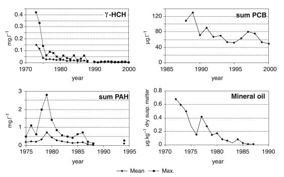
*Figure 5.* Yearly average concentrations of  $\gamma$ -HCH, sum PCB, sum PAH and mineral oil in the river Rhine measured at the German–Dutch border, including maximum observed concentrations of  $\gamma$ -HCH and sum PAH.
