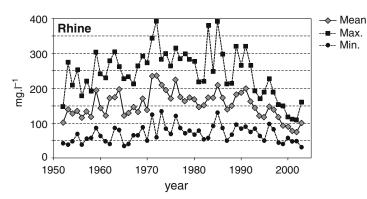
Figure 6. Yearly average, minimum and maximum observed chloride concentrations in the river Rhine measured at the German– Dutch border.
