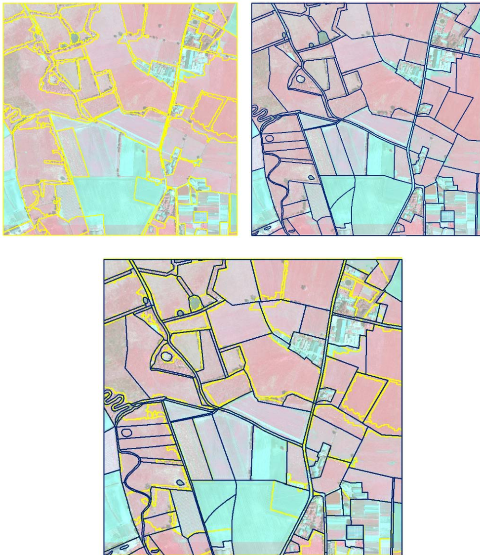
Figure 6 Visual comparison of semi-automated (yellow) and field based manual (blue) delineation of the habitat mapping units.
