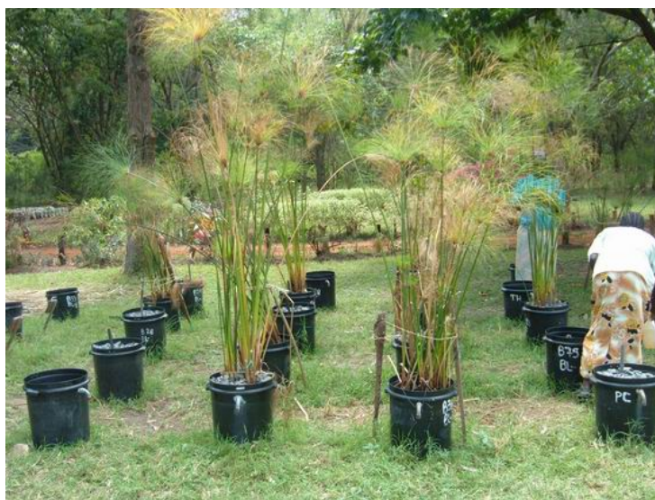
Fig. 6.2 Wetland bucket mesocosms used for study of phenol removal processes.
