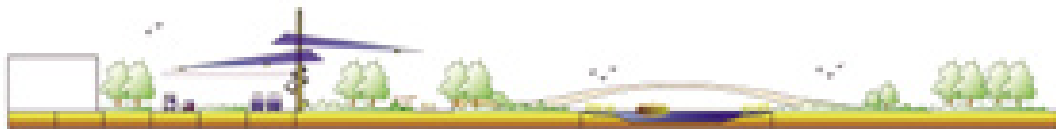
Fig 31: Profile A: main axis. Central axis of the Agropark with main canal with on its west side the infrastructural bundle, central pipeline bundle CPU with solar cell roofing and on the east side of the canal the landscape ecological zone.
