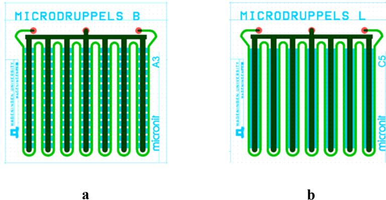
**Figure 3:** Parallelized EDGE systems ( $1.5 \times 1.5$  cm microchip) (a) EDGE-R (b) EDGE-W
