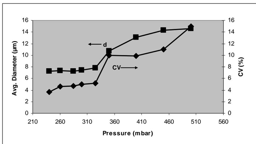
**Figure 2:** Average droplet diameter and CV as a function of applied pressure.
