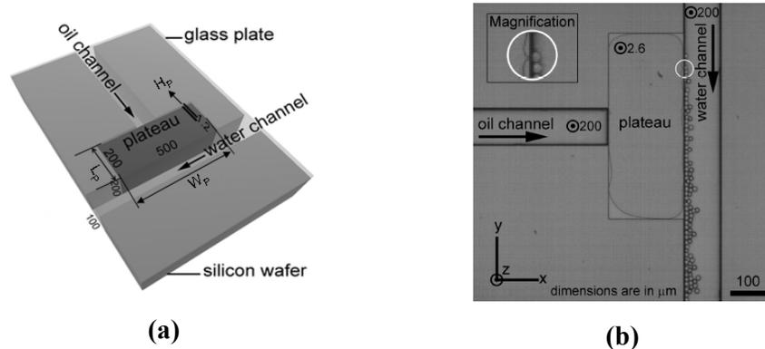
**Figure 1:** (a) Schematic three dimensional representation of a typical EDGE system (b) droplet formation through a typical EDGE device (van Dijke et al., 2010a).
