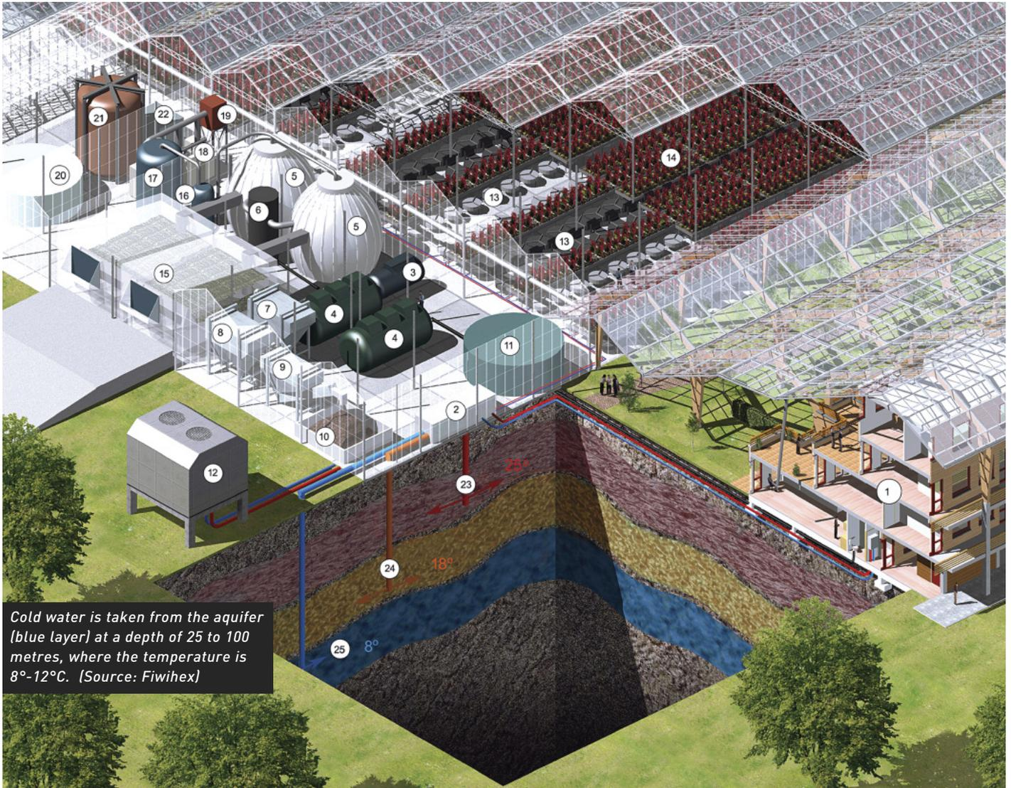
Cold water is taken from the aquifer (blue layer) at a depth of 25 to 100 metres, where the temperature is 8°-12°C. (Source: Fiwihex)
