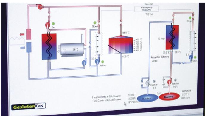
A computer screen depicting the heat and cooling of 'the closed greenhouse'.
