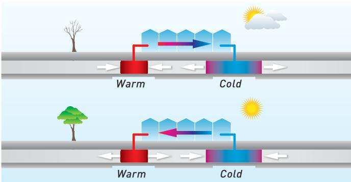
In summer, cold water from the aquifer is used for cooling. The water warms up and is stored. The tepid water can be used for heating in winter. (Source: Wageningen UR)
