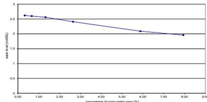
Figure 13. Percentage open water area versus water level in Don Bosco Compartment with the pumping capacity of 3 m<sup>3</sup>/s
