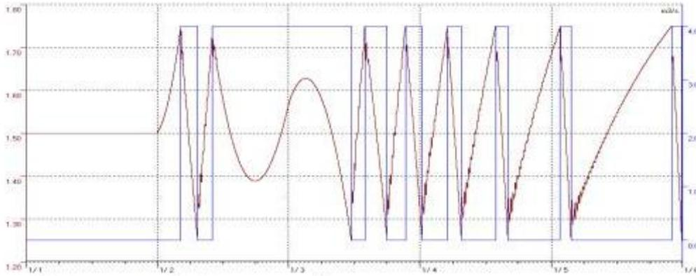
Figure 11. Water levels and pumping discharge at Don Bosco (3) Compartment
