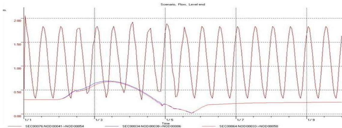
Figure 15. Water levels in Kelapa Gading influenced by land subsidence and sea level rise with increased pump capacity
