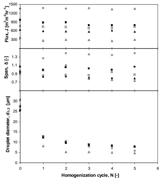
Fig. 3. Effect of particle size on droplet diameter and span, at a transmembrane pressure of 200kPa and bed thickness of 2.5mm: (○) support sieve, (Δ) 50 $\mu\text{m}$ , (▲) 63 $\mu\text{m}$ , (◻) 75 $\mu\text{m}$ , and (■) 90 $\mu\text{m}$
