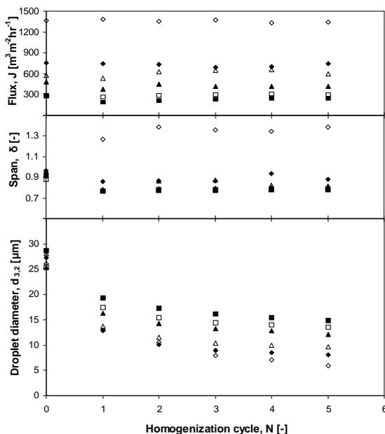
Fig. 2. Effect of bed thickness on droplet diameter and span, at a transmembrane pressure of 200kPa: (○) support sieve, (◆) 2.5mm, (Δ) 5mm, (▲) 10mm, (◻) 15mm, and (■) 20mm
