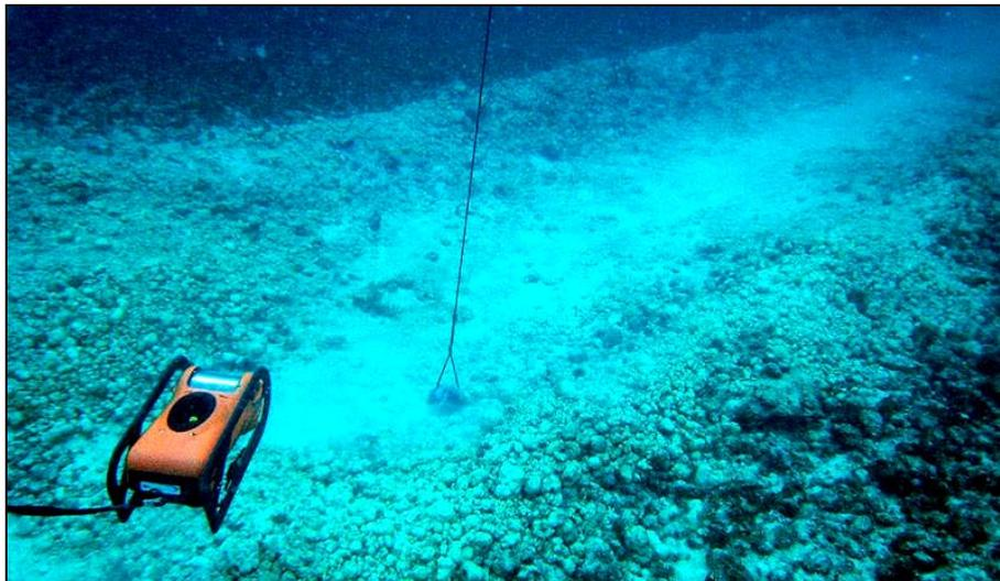
*Figure 15. Remotely operated vehicle exploring an anchor scar on the Saba Bank (source S. Lundvall).*
