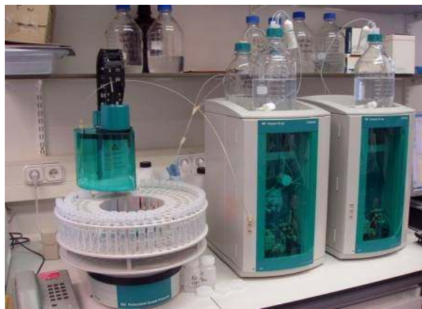
Figure 8: Ion Chromatography (IC) system, 850 Professional, Metrohm (Switzerland), for assessment of mineral composition in in-vitro propagated miscanthus plants
